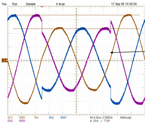
All three phases with 20ms dips, voltage 70%
