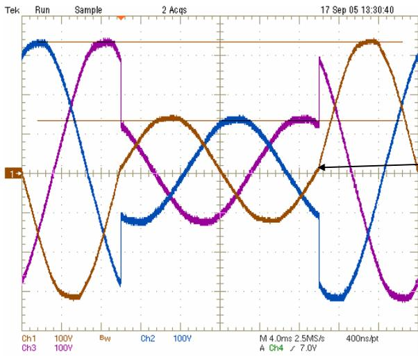
All three phases with 20ms dips, voltage 40%
