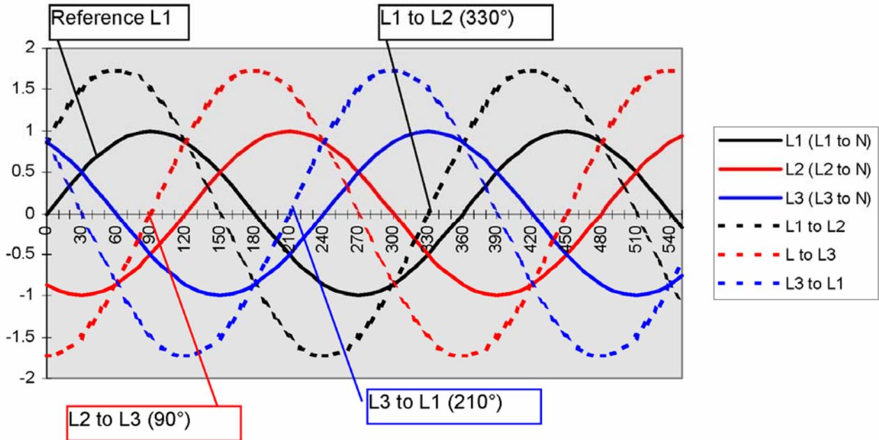
For all dips and interruption the zero crossing of L1 is the reference. The software calculate the phase shifting for L2, L3. The operator can select always the phase angle between 0 to 360° for each phase.
