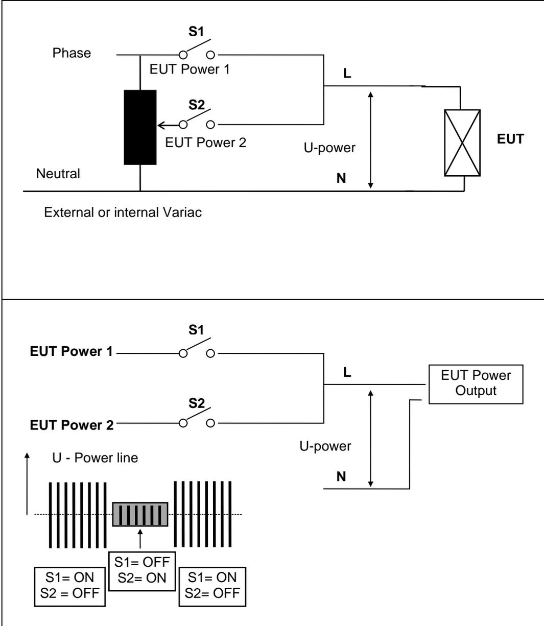
At DIPS to 0 % of the power line voltage, two operating conditions can be differentiated:
