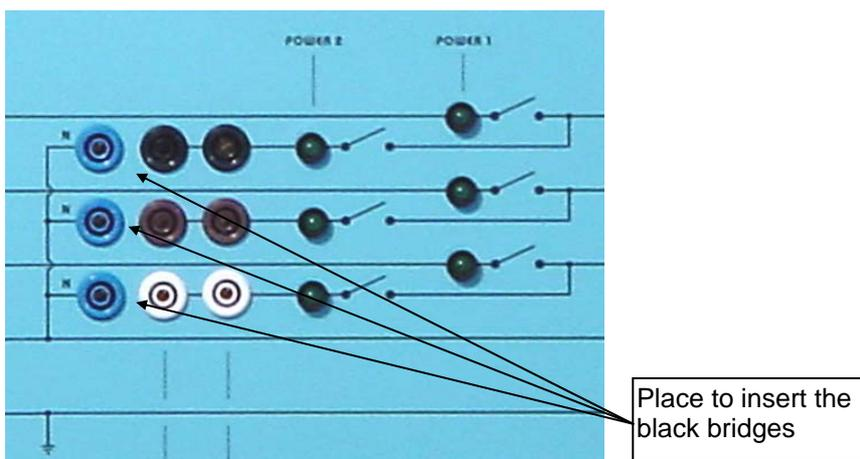
The different LED signalise in which phase the switching is activated. The Power 2 switch is used to connect the (SRC32) for dips simulation. When the three black bridges are inserted between phase to neutral, the power switch 2 can be used to simulate the High-Z mode.
