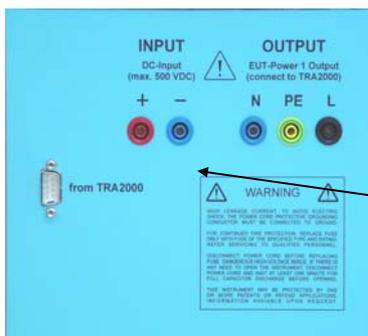
Connect the d.c. supply after you have removed the EUT Power1 cable on the rear side of the
