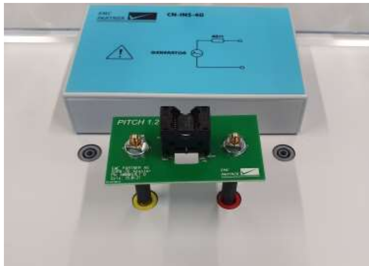
INS-SOP8-36 ADAPTER SET fitted directly onto generator high voltage outputs
