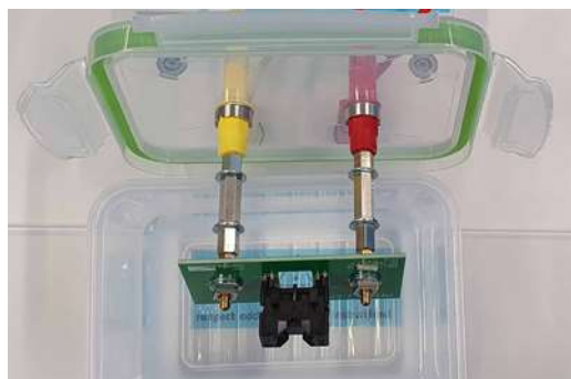
INS-SOP8-36 ADAPTER SET oil bath mounted on INS generator
