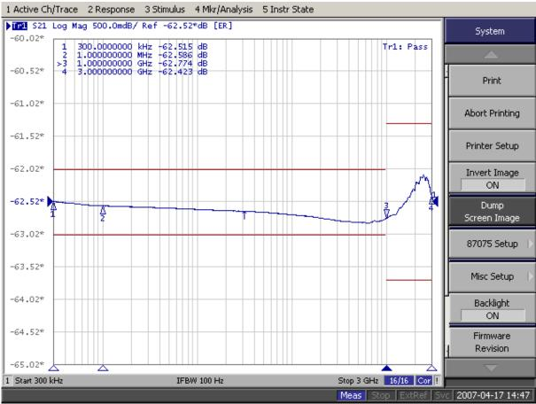
The target, attenuator and cable chain is over the frequency range within the tolerances. The nominal value is 42.17 or 62.52 dB +/-0.5dB up to 1 GHz and +/-1.2dB up to 4 GHz.
