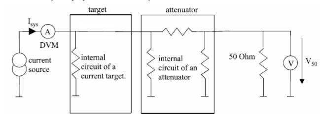
The low frequency system transfer impedance of the target - attenuator - cable chain can be determined by:
