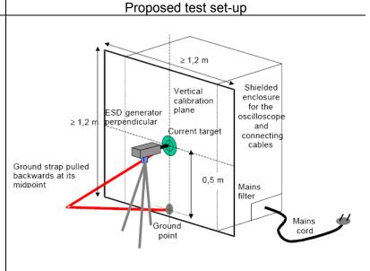
The target shall be mounted at the centre of the vertical calibration plane of at least 1.2m x 1.2m. The connection for the ESD generator return cable (ground strap) to the calibration plane shall be made directly below the target at a distance of 0.5 below the target. The ground strap shall be pulled backwards at the middle of the cable, forming an isosceles triangle. It is not allowed to let the ground strap lay on the floor during the calibration.
