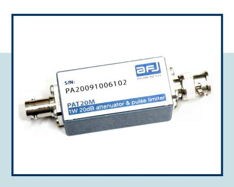
This 20dB attenuator is designed for pulse voltages up to 1Ws, to protect the input receivers. Even using EMI Test systems already protected against spikes, for unknown devices under test, the PAT 20M pulse limiter is strongly recommended.
