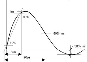
Both waveforms are verified in open circuit (voc)and short circuit (isc).
