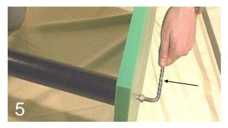
Assembly the first tube with the stand plate. Tighten the screw and place the tube in vertical position.
