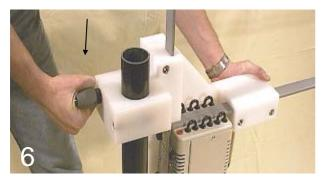
Put the antenna onto the first tube and fix it by tightening the black handle.
