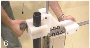
Put the antenna onto the first tube and fix it by tightening the black handle.
