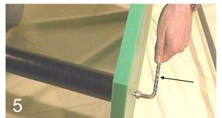
Assembly the first tube with the stand plate. Tighten the screw and place the tube in vertical position.
